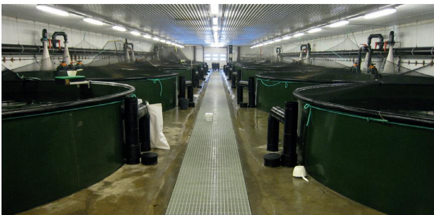
*Figure 1.1 An indoor recirculation system.*
