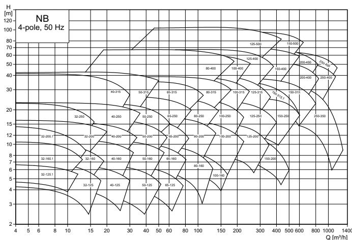
*Figure 2.19 Centrifugal pumps type NB for pumping water when high pressure or high lifting heights are needed. The range of centrifugal pumps is wide, so these pumps are also efficiently used for pumping at lower lifting heights. Centrifugal pumps are often used in recirculation systems for pumping secondary flows as for example flows through UV systems or for reaching high pressure in oxygen cones. H is the lifting height and Q is the volume of water lifted.*
