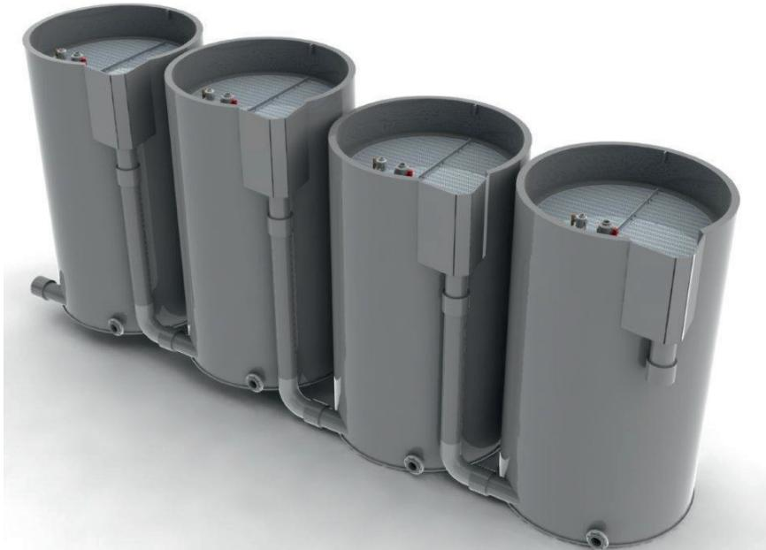
*Figure 5.6 The flow pattern in the shown multi chamber PE biofilter goes from left to right and upstream in each chamber. Most of the organic material is removed by heterotrophic bacteria in the first chamber. The consequent low organic load in the latter chambers secures a thin nitrifying biofilm for converting ammonia to nitrate. The last chamber is called a microparticle filter and is designed for removal of very fine particles that have not been removed by the mechanical filter.*
