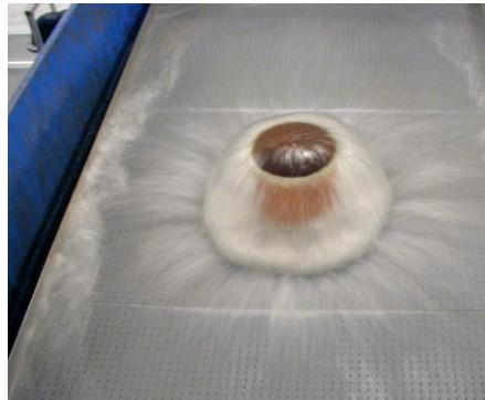
*Figure 5.1 Water quality and flow in filters and fish tanks should be examined visually and frequently. Water is distributed over the top plate of a traditional trickling filter (degasser) and distributed evenly through the plate holes down through the filter media.*
