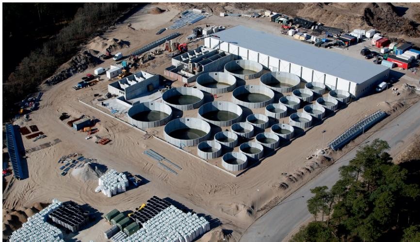
*Figure 8.5 A 2 000 tonnes salmon farm in Hirtshals, Denmark under the construction phase in 2013. The system is based on recirculation technology and is covered by a building for completion to control temperature and have high biosecurity. Salmon are grown from eggs to 4 kg size in 2 years in large tanks reaching almost 1 000 m<sup>3</sup> each. The white bigbags in the foreground are packed with biomedia ready for installation in the biofilter chambers. Source: Axel Søgaard/AKVA group.*
