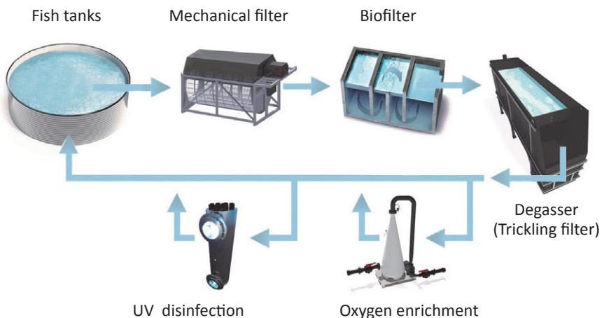
*Figure 2.1 Principle drawing of a recirculation system. The basic water treatment system consists of mechanical filtration, biological treatment and aeration/ stripping. Further installations, such as oxygen enrichment or UV disinfection, can be added depending on the requirements.*
