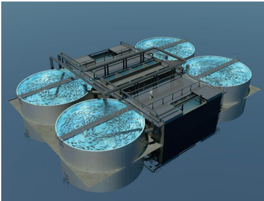
*Figure 8.6 Recirculation systems become increasingly larger with bigger tanks to accommodate for increasing production volumes. Shifting smolt sizes in Norway from 100 gram to 300 gram will triple the land based production, thus current Norwegian smolt production on land of around 35 000 tonnes per year will increase to around 100 000 tonnes.*
