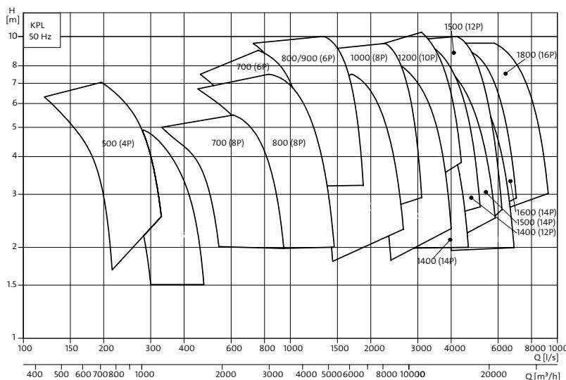
*Figure 2.18 Lifting pumps type KPL for efficient lifting of large amounts of water. Lifting pumps are often used for pumping the main flow in the recirculation system. Correct selection of pump is important to keep the running costs down. Frequency control is an option to regulate the exact flow needed depending on the fish production. H is the lifting height and Q is the volume of water lifted.*
