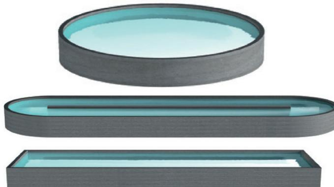
*Figure 2.6 Circular tank, D-ended raceway, and raceway type.*
